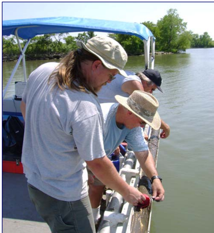
Kansas Biological Survey scientists Matt Linden, Scott Campbell, and Jerry deNoyelles (l. to r.) examine a sediment core extracted from Winfield City Lake. The lake is one of numerous reservoirs around the state being mapped and cored by KBS's Applied Science and Technology for Reservoir Assessment (ASTRA) Initiative, funded by the State Water Plan Fund through a contract with the Kansas Water Office.
