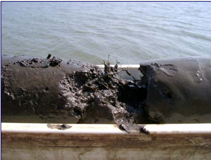
Distinguishing between the original lake bottom and the accumulated sediment is relatively easy. The original substrate (left) is tightly packed and has coarser soil particles. A transition zone of old vegetation (center) separates it from the finer grained sediment (right).
