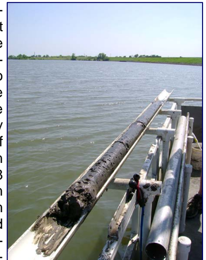
Core samples help validate the information obtained by using state-of-the-art mapping sonar to measure lake depth and the thickness of sediment deposits.
